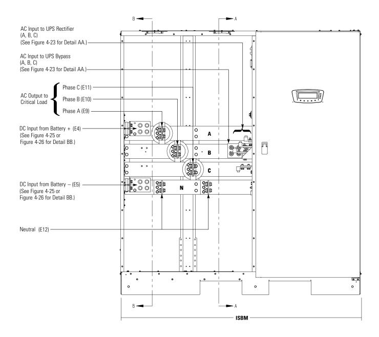
Figure 4-22. ISBM Section Power Terminal Locations – Separate Rectifier Feed
